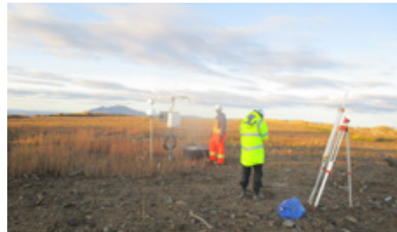
/ Collecting data from dedicated weather stations situated on the Platinum Gulch Waste Rock Storage Area to further reclamation and closure research on the Project.
